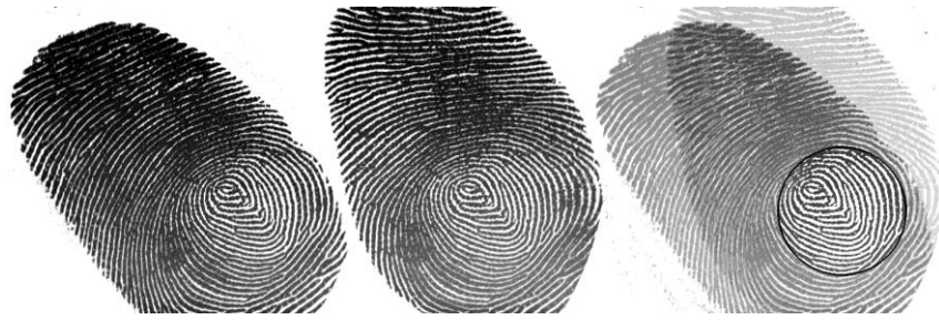
Figure 22: Two different impressions of the same fingerprint before and after best registration.
