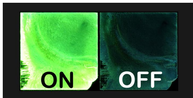
Figure 3. Fluorescence images of M2 nanoparticle film spin-casted on the glass substrate (a) before and (b) after exposure to THF vapors for 3 min. The photos are taken under UV excitation.
