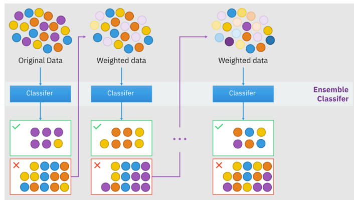
Figure 4: Figure represents the concept behind boosting [2]. Multiple learners are generated each improving the classification based on previous learners, which are called weak learners.
