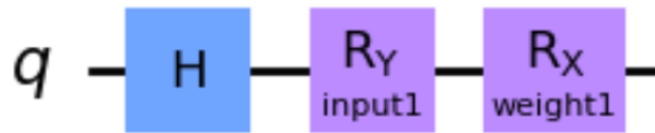
Figure 1: Figure shows a single qubit quantum circuit with a Hadamard gate, and input & weight parameters.
