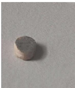
Figure 4. SGDC-1500-2h-cp sample with platinum electrodes, 2.9mm diameter, 1.45mm height.
