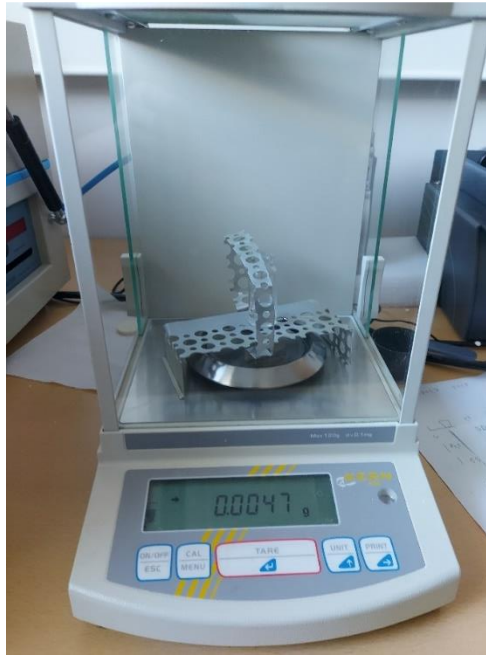
Fig. 2. Setup for measuring mass of pellets in acetone. Bottom stand is used to hold vial with acetone, top stand is used to keep pellet submerged in acetone and not to touch the vial. Top stand stands on scales and is compensated.
