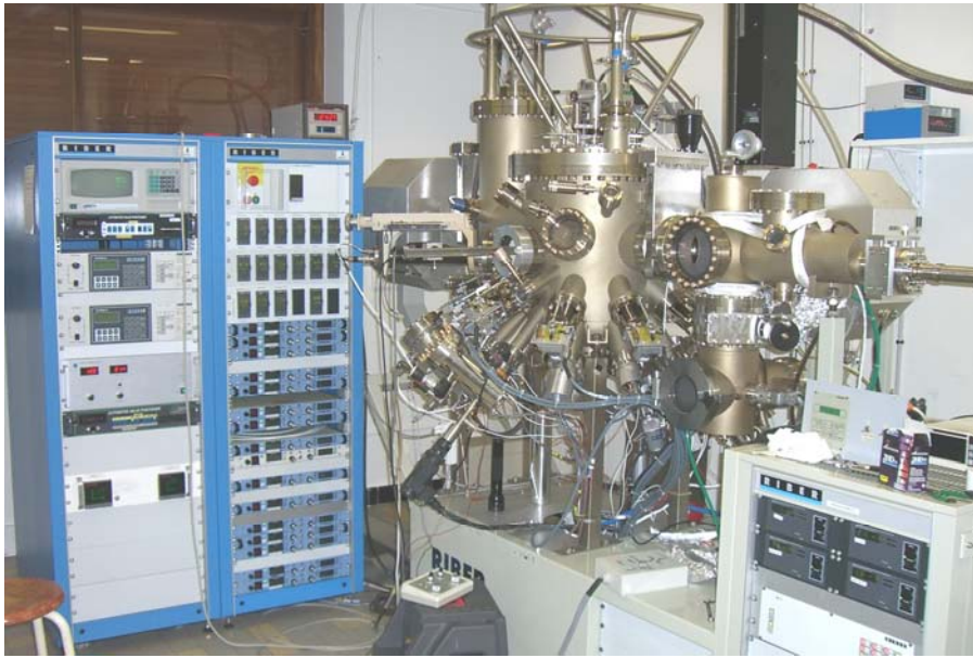
Figure 2.2: Photo of the RIBER Compact 21E MBE machine used for the growth of QCL wafers.
