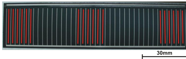
Fig. 84 Red lines indicate laser scribed trenches in complete single cell. The total length of the scribes was 360 mm.
