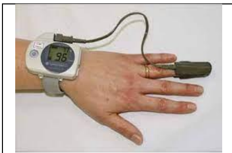
Figure 2. Finger pulsoxymetry with data memory for nocturnal saturation measurement or for stress tests.
