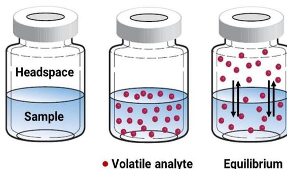
**Fig. 12.** Sealed headspace vial used for sample introduction into GC system.
