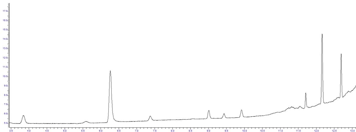
**Fig. 21.** Chromatogram of the selected ORSs, at a concentration of 5 ppm.
