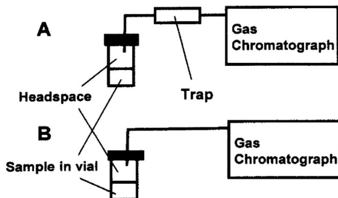
**Fig. 13.** Dynamic vs. static headspace sampling technique. (A) Dynamic headspace uses a trap to concentrate and collect volatile residual solvents before introduction to the column. (B) static headspace technique in which a volume of the headspace gas phase is introduced directly to column [78].
