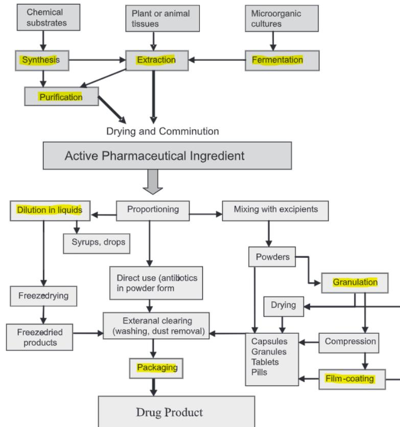
**Fig. 10.** An illustration of general selected manufacturing process in pharmaceutical industry, the highlighted boxes represent the steps which can be potentially contaminated by organic solvents [61].
