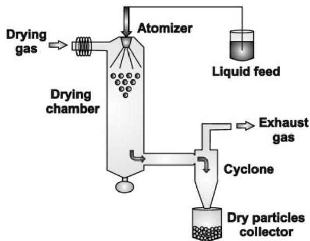
**Fig. 11.** An illustration of spray drying process in pharmaceutical industry [69].
