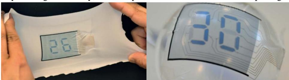
*Figure 3. PEDOT:PSS based fully printed stretchble double seven segment display. Deposited onto textile and displaying number 26 (left), display compeletly adhearing to round suraface due to its stretchability (right) [20].*
