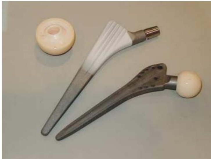
Fig. 3. Calcium phosphates in hip endoprostheses: a ceramic ball joint ( \text{Al}_2\text{O}_3 ), a calcium-phosphate coated endoprosthesis („cementless endoprosthesis“), and an uncoated endoprosthesis that must be fixed in place with PMMA bone cement [2].
