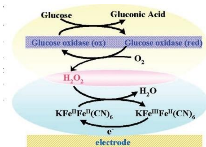
Fig. 9. Schematic representation of the application of PB for the multilayered biosensor [56].
