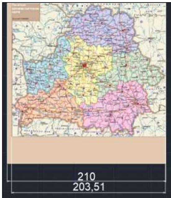
Fig. 3.10. Bringing the Political-Administrative map of the Republic of Belarus to the scale of the printed version and measuring the size of the study area.
