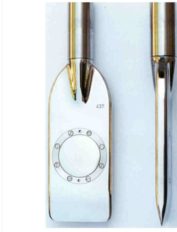
3.3 pav. Dilatometro mentelė ( https://www.marchetti-dmt.it/dmt-instrumentation )
