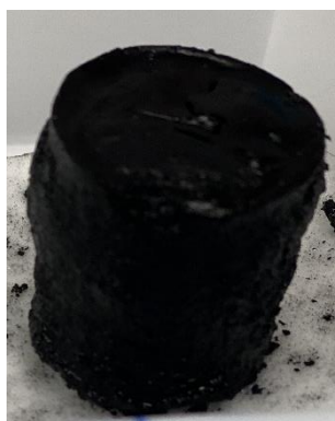
Fig. 2.1. Sponge-like NS-G prepared by hydrothermal analysis
