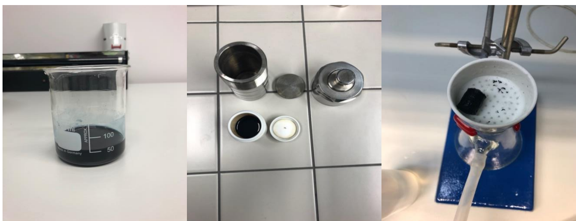
Fig. 5. Modification of GO with dyes. (a) GO +MG after sonification. (b) Transfer of mixture into teflon autoclave. (c) Filtration of GO + MG.
