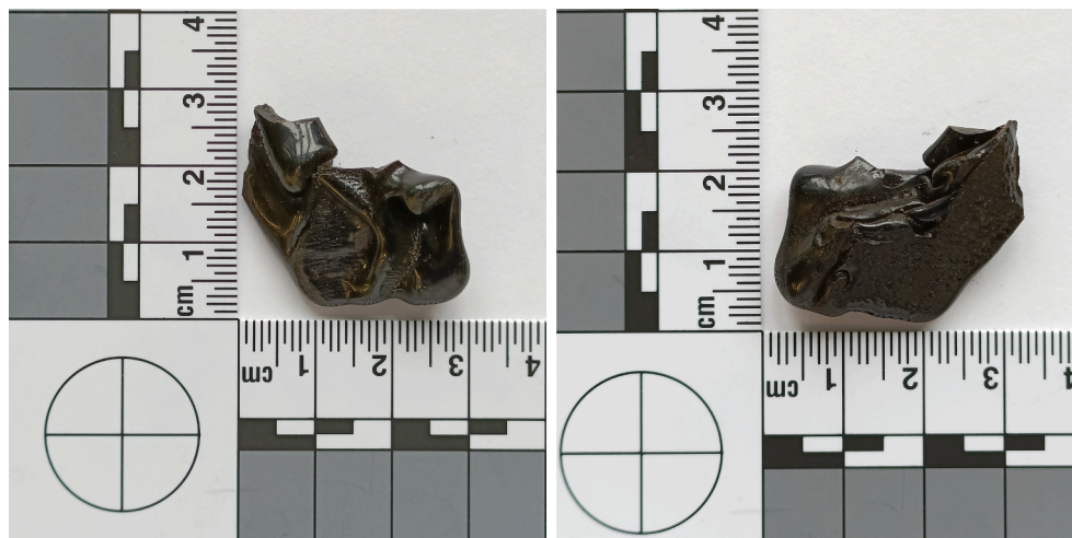
Fig. 2. Resin sample. Left: upper surface showing flow patterns, right: lower surface showing pattern of wooden surface.
