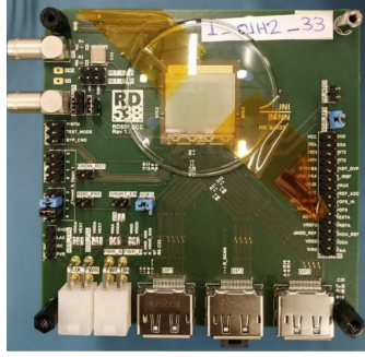
Figure 2: A CROC_v1 chip (under the transparent cover) mounted on the single-chip card (green).
