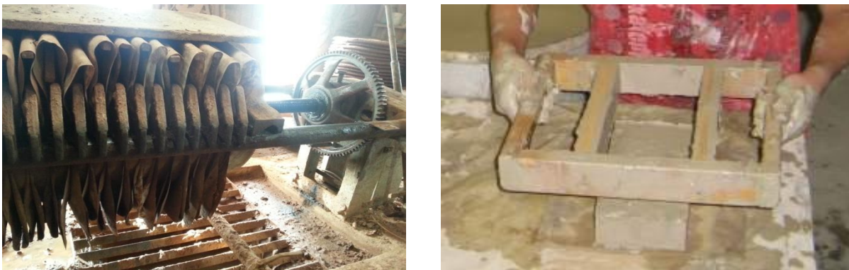
Fig. 14. The expression of water from milky clay (on the left) and the formation of clay bricks with the help of wooden frames (on the right).
