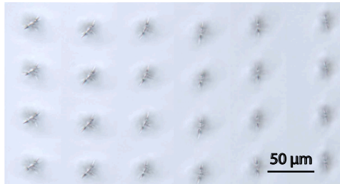
Fig. 10. Directional cracks obtained with the Airy binary beam inside EXG glass. The rotation of the GPE changed by 15 degrees every column. Microscope picture of a single plane. Modifications made with 10 ps, 290 μl pulses.
