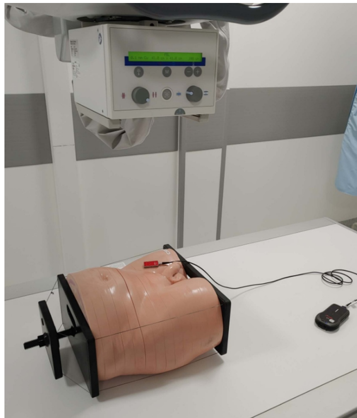
Figure 1. Experimental setup to simulate pelvis x-ray examinations with CIRS phantom.
