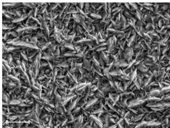
Fig. 24. SEM image of pure Co electrodeposited from the citrate baths.
