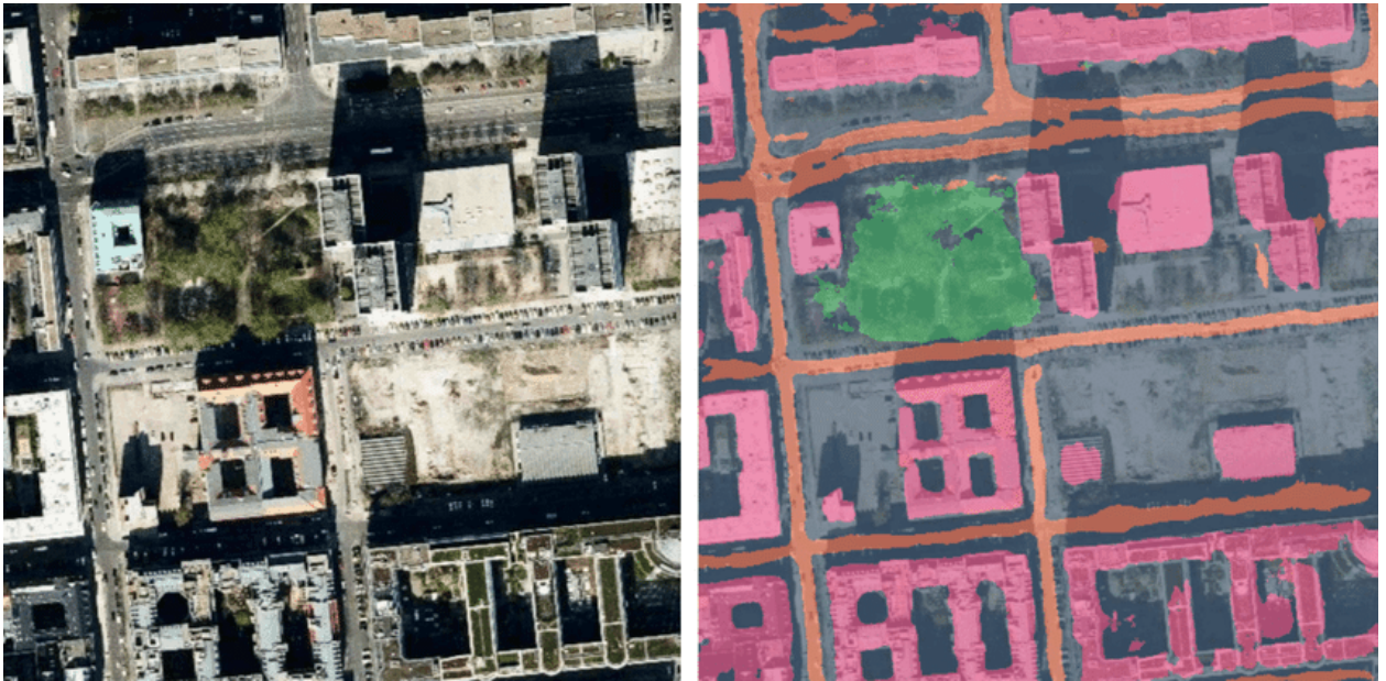
Figure 1. Left: Image taken from an earth-orbiting satellite. Right: Same image with semantically segmented roads, buildings and vegetation. (photo taken from [NH18])
