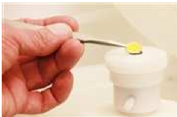
Fig. 2.10. Quartz sensor with gold surface, provided by Q-Sense® and used in the research.
