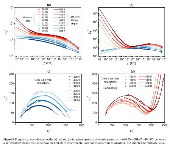
at different temperatures. Lines show the best fits of experimental data points according to equation (2). Complex permittivity (Cole-Cole) plots for (c) low and (d) high temperature ranges, illustrating the thermally-activated conduction losses.
