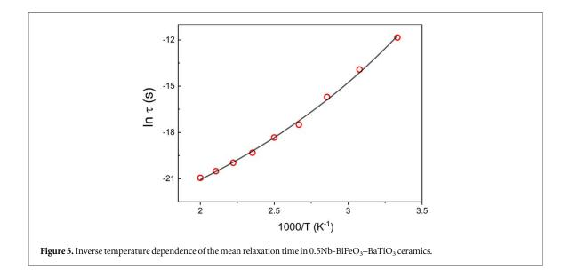
Debye-type dispersion ( $\alpha = 0$ ) where only one type of dipole causing one relaxation time exists. Another parameter, the strength of the relaxation,  $\Delta \varepsilon$ , clearly shows the opposite trend with respect to temperature compared with parameter  $\alpha$ . This implies a decreasing contribution to the total dielectric permittivity of this relaxation process on cooling.
