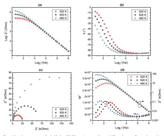
**Figure 2.** Impedance spectroscopy data for Nb-doped BF-BT ceramics presented in several different formats to illustrate the transition from a predominantly capacitive ( $\phi < -45^{\circ}$ ) to resistive ( $\phi > -45^{\circ}$ ) electrical response at low frequencies and higher temperatures. Bode plots for (a) impedance magnitude and (b) phase angle; (c) complex impedance plot; (d) bode plots for imaginary parts of complex modulus and impedance.
