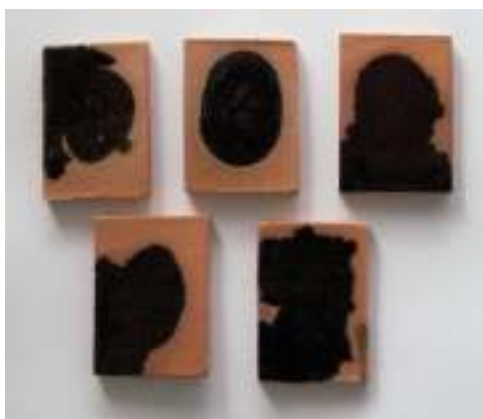
Fig.16. The pictures of black ceramic glazes obtained using nanoferrites: \text{YFeO}_3 (top, left), \text{Y}_3\text{Fe}_5\text{O}_{12} (top, middle), \text{ZnFe}_2\text{O}_4 (top, right), \text{NiFe}_2\text{O}_4 (bottom, left) and \text{CoFe}_2\text{O}_4 (bottom, right).
