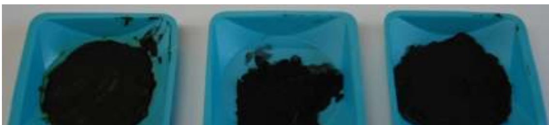
Fig. 2. The picture of black oily colorants produced from C soot and \text{CaCO}_3 having different ratios (from left): 1:1; 1:0.1 and 1:0.01.
