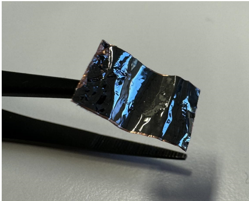
Figure 29: Exfoliated flexible membrane on sticky conductive copper tape.
