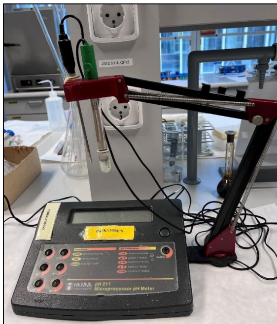
4 pav. pH registravimui naudotas jonometras Hanna Instruments Microprocessor pH Meter pH 211
