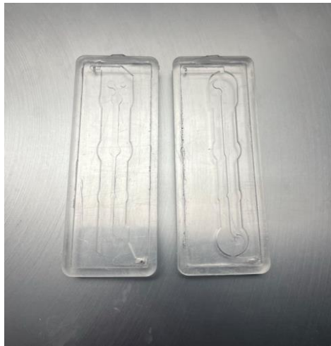
Fig. 2.3 PDMS masters. Bottom and top parts shown on the right and left sides, respectively (Photo courtesy of the author).
