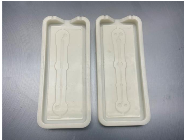
Fig. 2.2 Completed 3-D printed master molds for lab-on-a-Chip fabrication. Bottom and top parts shown on the left and right sides, respectively (Photo courtesy of the author).
