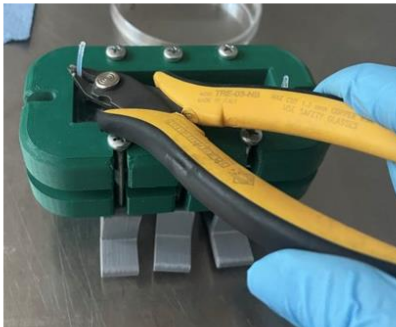
SFig. 5. Half of the inlet and outlet hoses are cut with pliers. (Photo courtesy of the author).
