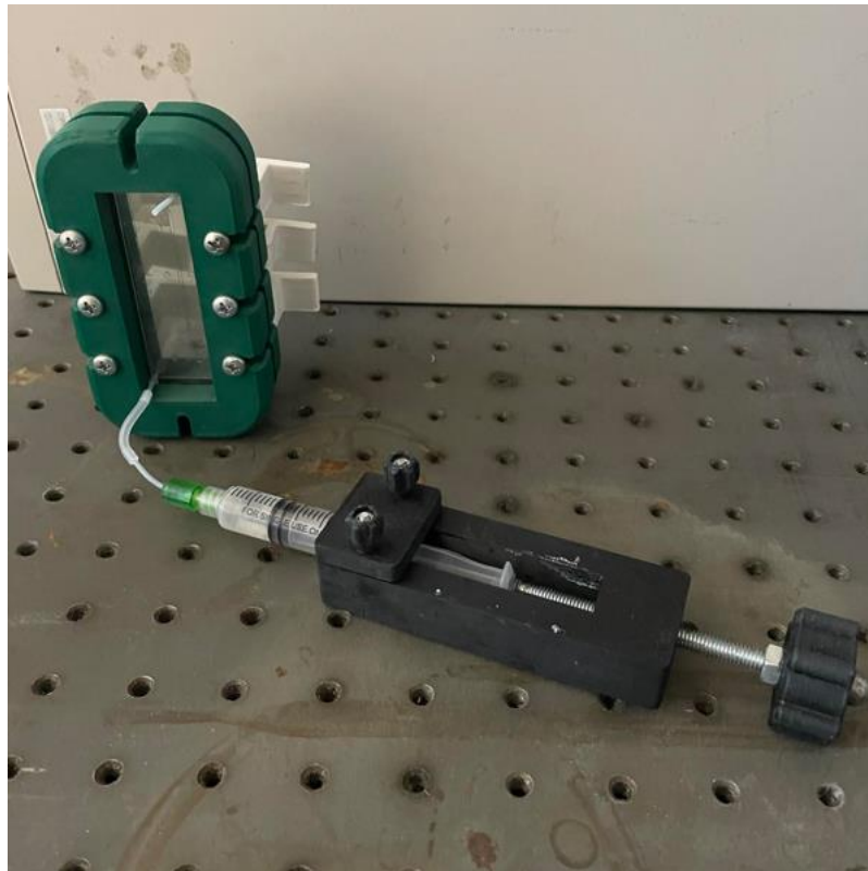
SFig. 4. Syringe holster connected to constructed apparatus. (Photo courtesy of the author).
