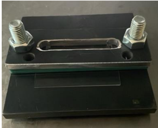
SFig. 15. High pressure clamping and curing jig assemble. (Photo courtesy of the author).
