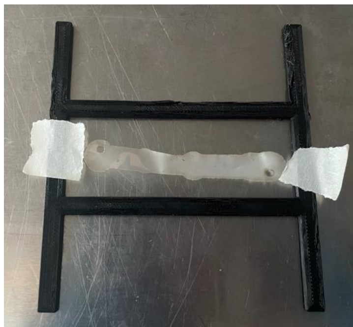
SFig. 7. Polycarbonate membrane on the special frame. (Photo courtesy of the author).
