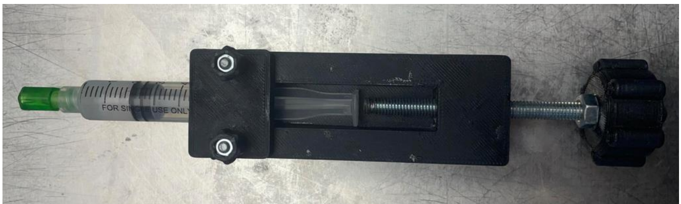
SFig. 1. Syringe with prepared OSTE in syringe holder. (Photo courtesy of the author).
