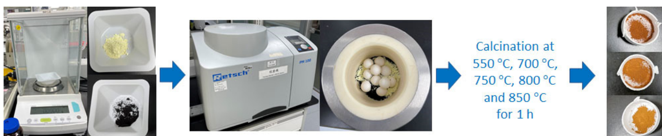
Figure 1. Solid-state reaction synthesis of \text{Bi}_{25}\text{FeO}_{40} .
