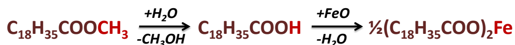
Figure 1.7. Formation of free fatty acid in biodiesel through hydrolysis and metal soaps
