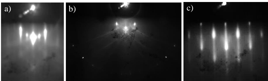
Fig. 4.1.3 RHEED images of the flat \text{SrRuO}_3 film surface a), of atomically smooth \text{SrTiO}_3 substrate b) and 3D diffraction from islands on the \text{SrTiO}_3 doped with Bi film surface c) (experiments in EPFL LC).
