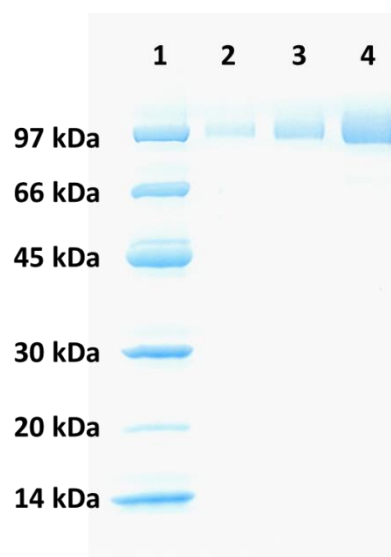
Figure 30. SDS-PAGE of HiCDH . Line 1 - molecular mass rulers; lines 2-4 correspond to HiCDH preparations (0.6 µg, 1.3 µg, and 2.5 µg, respectively) applied on SDS-PAGE.
