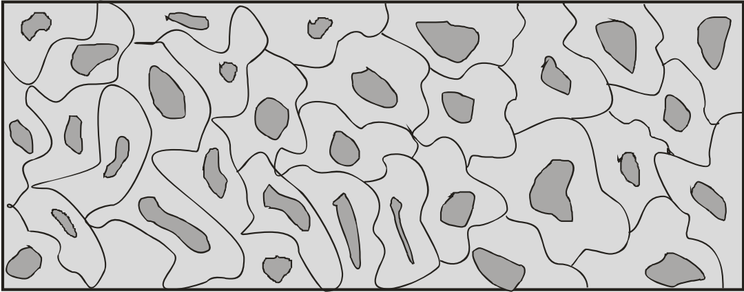
Fig. 1.4 Mixed phase materials of Maxwell Garnet effective medium model.
