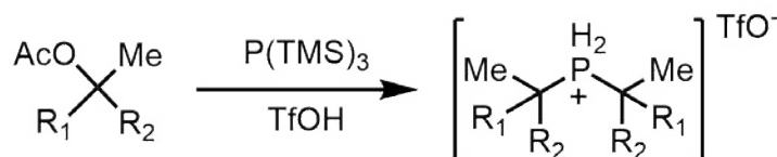
Fig. 1. Synthesis of di- tert -alkyl phosphine salts using P(TMS) 3
