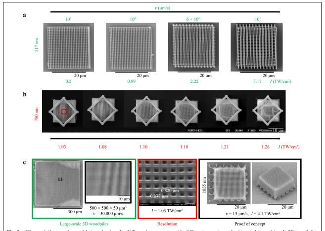
Fig. 3 a 3D woodpiles are shown fabricated using the 517 nm laser source with different scanning velocities and intensities. b 3D woodpiles developed with the 780 nm laser source with a scanning speed at 30  $\mu$ m/s while the power is altered from 20.5–25 mW. c The fabrication highlights of the non-photosensitized SZ2080<sup>TM</sup> are presented for 1035 nm (black frame), 780 nm (red frame) and 517 nm (green frame).
