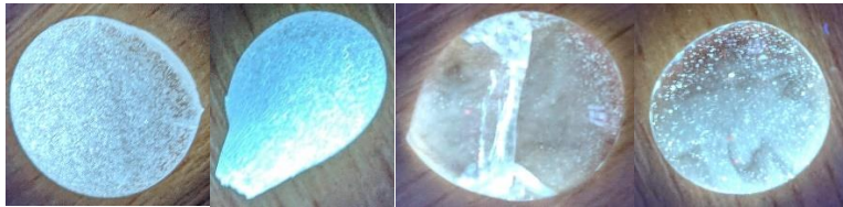
Figure 18. Examples of as synthesized glasses showing inhomogeneous distribution of glass components within finished samples.
