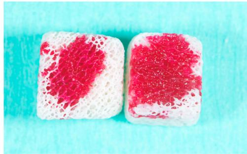
**Figure 5.** Top view of a sample. Great wettability after three time cycles (right sample) of vacuum plasma surface treatment.
