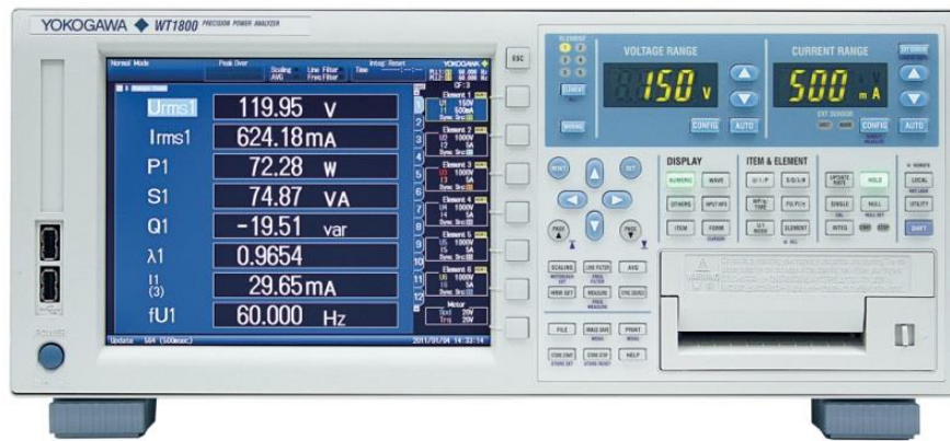
Figure 1.2.3. Yokogawa WT1800 – Power Analyzer.
