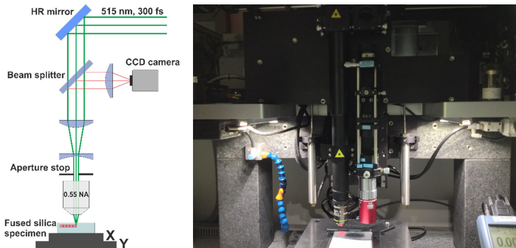
Figure 10 Optical design of the laser micromachining system (left) and laser micromachining system picture (right).
