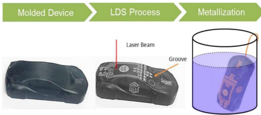
Figure 13. LDS process steps [91].
