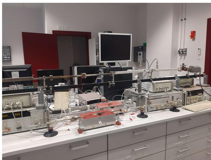
**Figure 1.** Setup for microwave dielectric measurements.
