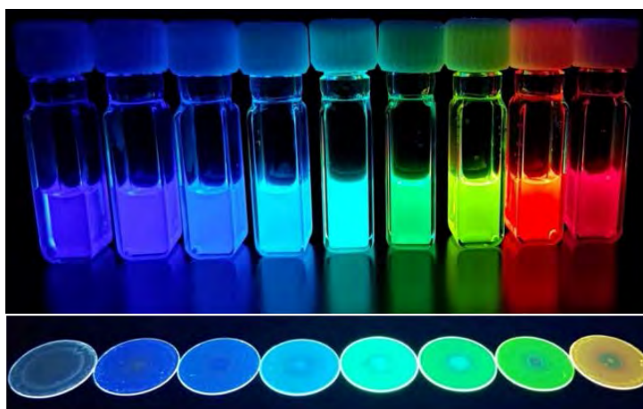
Fig. 1. Color gamut of obtained multicolor PQDs in toluene (top) and immobilized in polymer matrix (bottom) under UV excitation ( \lambda_{ex} 365 nm).
