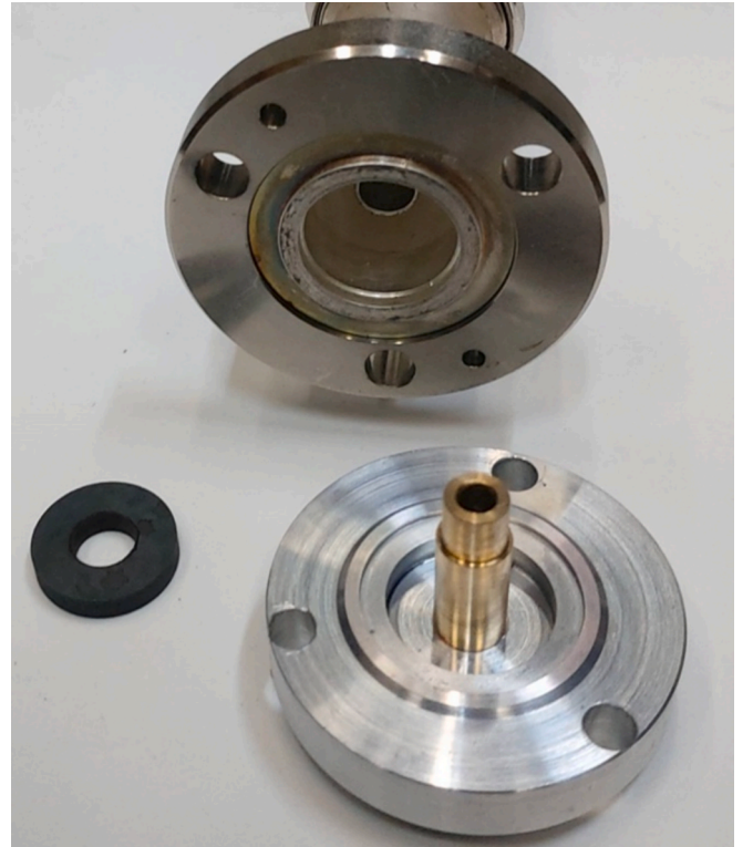
Fig. 3. Measurement setup using single-turn inductor method for AL-800 ferrite, with a standard 7/8 coaxial line.
