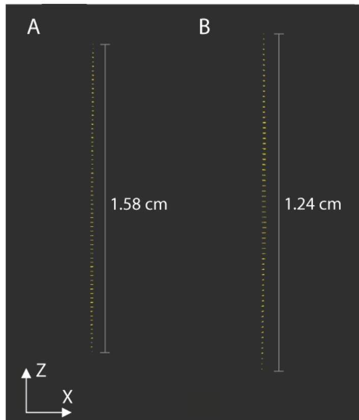
**Figure 17** Visualising the intensity distributions. A – 1 px phase mask. B – 10 px phase mask.
