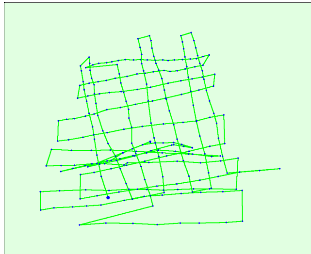
Figure 2: Top view of the initial image position. The green line follows the position of the images in time starting from the large blue dot.
