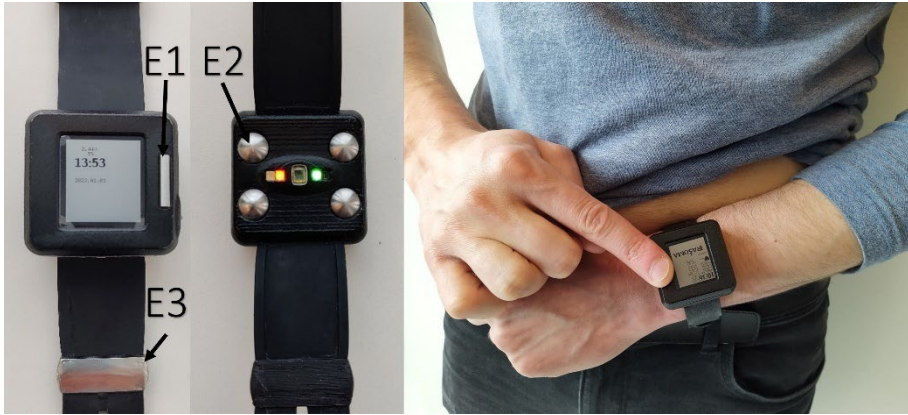
Figure 4. Prototype of the wearable device (left panel); acquisition of a 6-lead ECG without any wires (right panel).
