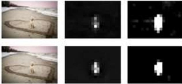
Figure 2.4: DeepLabV3 (first row) and FCN (second row) results, using 294 30 \times 30 occlusions. Min-max normalized maps are in the second column while z-score standardized maps are in the third. Either one of these techniques can be used to generate more color intensities in the final explanation.
