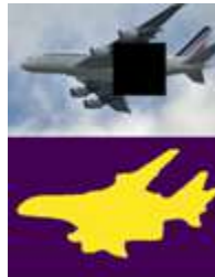
Figure 3.4: The occluded airplane fuselage and the corresponding output, generated by FCN.
