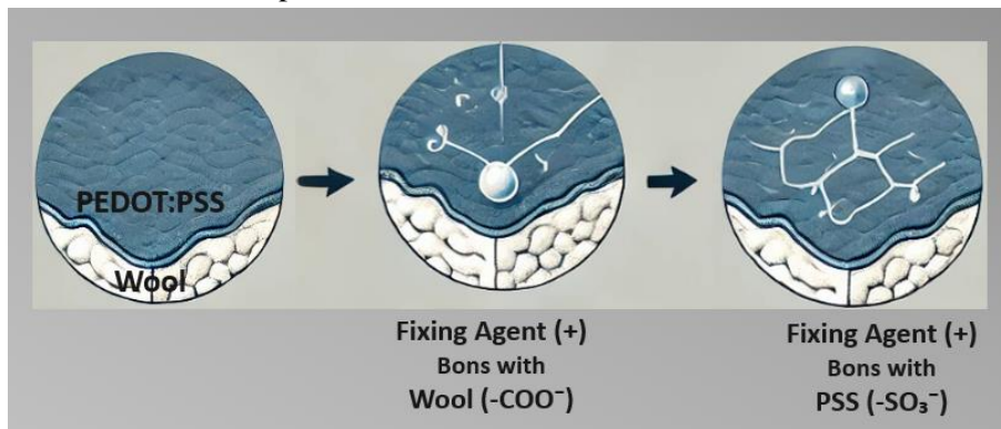
Figure 28. Tubicoat fixing agent HT as a bridge between wool and PEDOT:PSS Tubicoat fixing agent.
