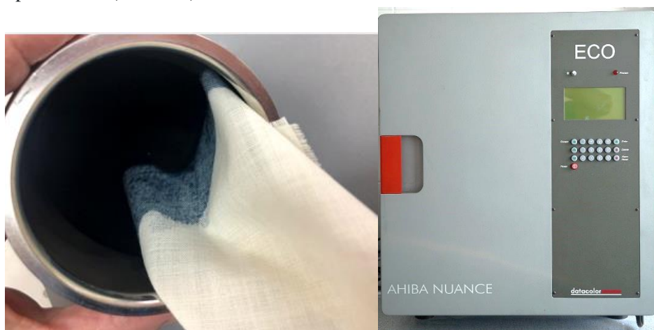
Figure 7. Wool fabric sample immersed into PEDOT:PSS water dispersion (a), views of cups in laboratory dyeing device, Ahiba Nuance ECO (b).
