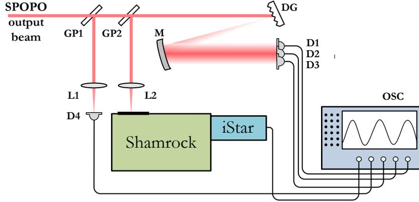
Figure 3.1 Detection setup. GP1 and GP2 – UVFS glass plates, DG – diffraction grating, L1 and L2 – lenses, M – large aperture mirror, D1 – D4 – fast photodiodes, Shamrock – spectrograph, iStar – intensified CCD camera, OSC – oscilloscope.
