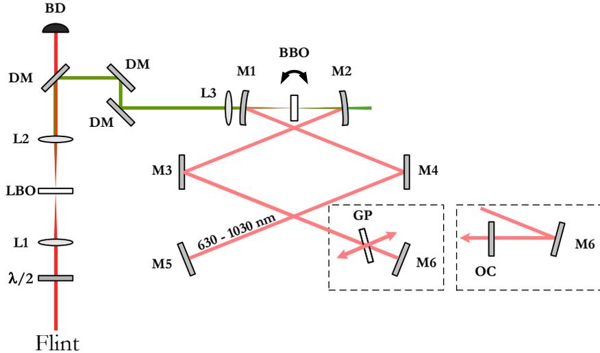
Figure 1.1 Experimental setup. Flint – Yb:KGW oscillator;  $\lambda/2$  – half-wave plate; L1 - L2 – lenses; LBO – lithium triborate nonlinear crystal; DM – dichroic mirrors; L3 – triplet lens; M1 and M2 – meniscus mirrors; BBO –  $\beta$  – barium borate crystal, M3 - M6 – complementary chirped mirror pairs; GP – glass plate; OC – output coupler.
