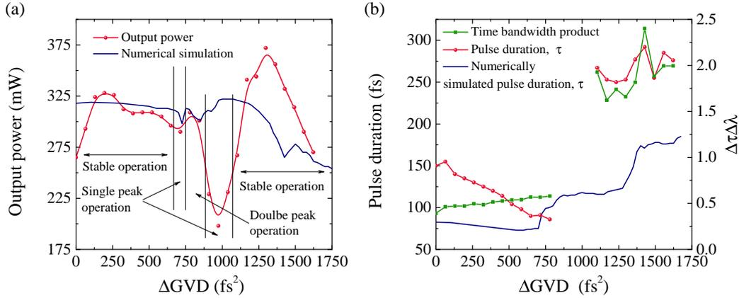
Figure 3.4 (a) SPOPO output power, (b) pulse duration and time bandwidth product dependence on  $\Delta\text{GDD}$ . The points depict experimental data, whereas the solid lines represent a cubic spline added to guide the eye.
