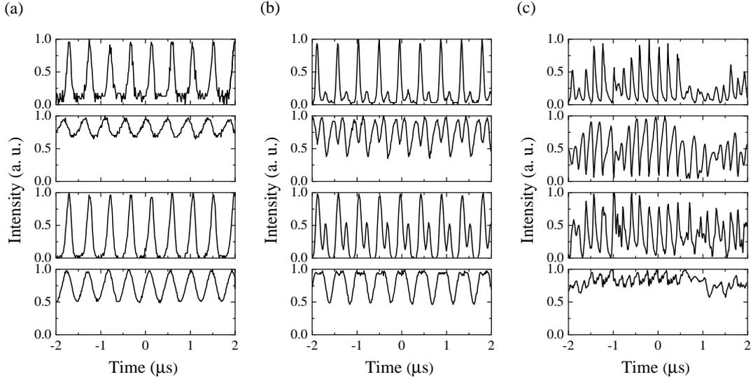
Figure 3.2 Amplitude of different spectral components (top row at 679 nm, second from the top 695 nm, third from the top at 706 nm) and overall energy (bottom row) variation at 1.7 W (a), 2.15 W (b) and 3.05 W (c) pump powers.
