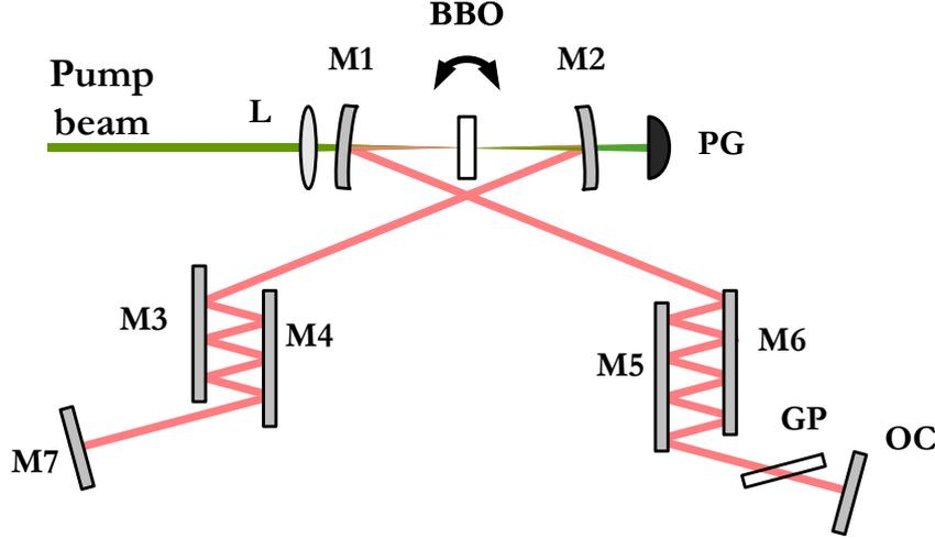
Figure 2.1 Experimental setup. L – triplet lens; M1 and M2 – meniscus mirrors; BBO –  $\beta$  – barium borate crystal, M3 – M6 – complementary chirped mirror pairs; M7 – flat broadband mirror, GP – glass plate; OC – output coupler.
