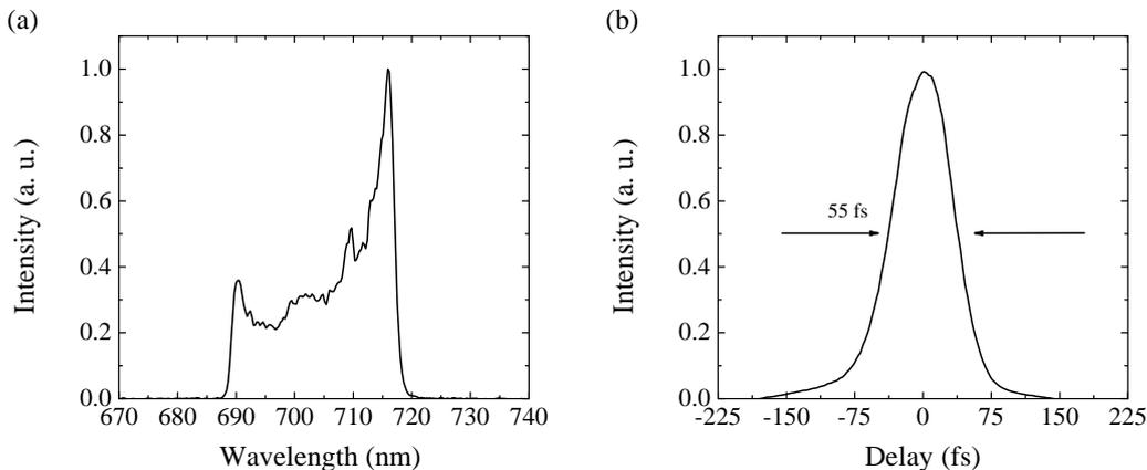
Figure 3.5 (a) Output spectrum generated in the SPOPO cavity without dispersion compensating prisms and (b) measured autocorrelation function.
