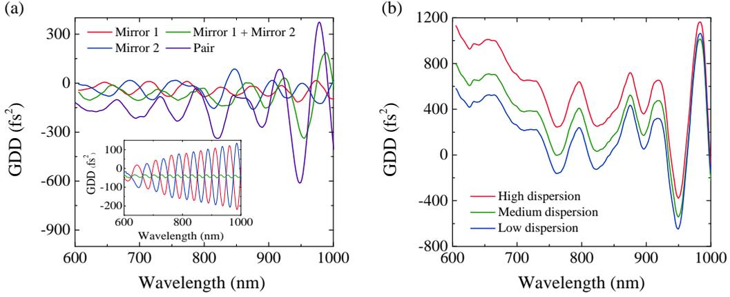
Figure 1.2 (a) Experimentally measured GDD of complementary chirped mirrors measured at 0 deg angle and GDD of chirped mirror pair measured at  $\sim 9$  deg angle of incidence. Inset shows designed GDD curves. (b) Cavity round trip GDD for high, medium and low dispersions SPOPO cavity configurations.
