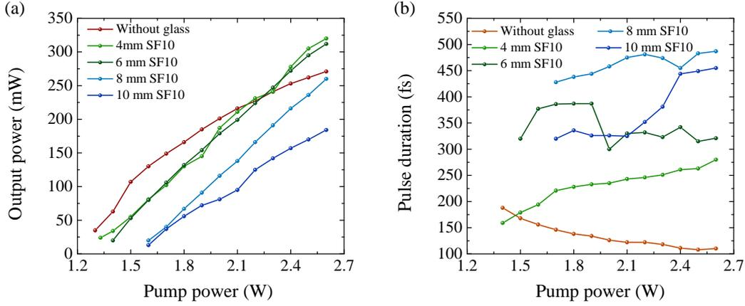
Figure 2.4 (a) Output power and (b) pulse duration dependence on pump power in the case of various SPOPO cavity arrangements.
