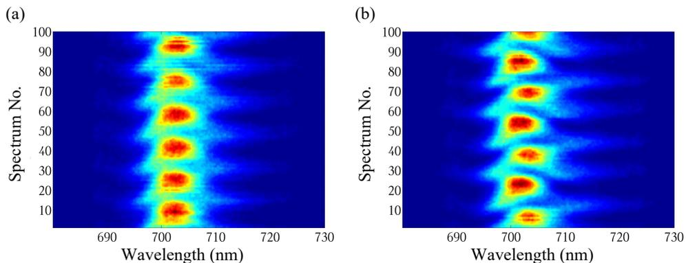
Figure 3.3 Sequences of SPOPO output spectra recorded with intensified CCD camera at 2.7 W (a) and 2.9 W (b) pump power.
