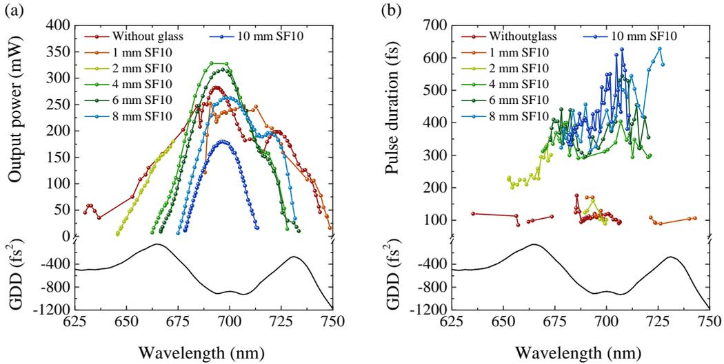
Figure 2.3 (a) Output power and (b) pulse duration dependence on signal wavelength in the case of various SPOPO cavity arrangements. Intracavity dispersion of the SPOPO without a glass plate is given at the bottom of the pictures.
