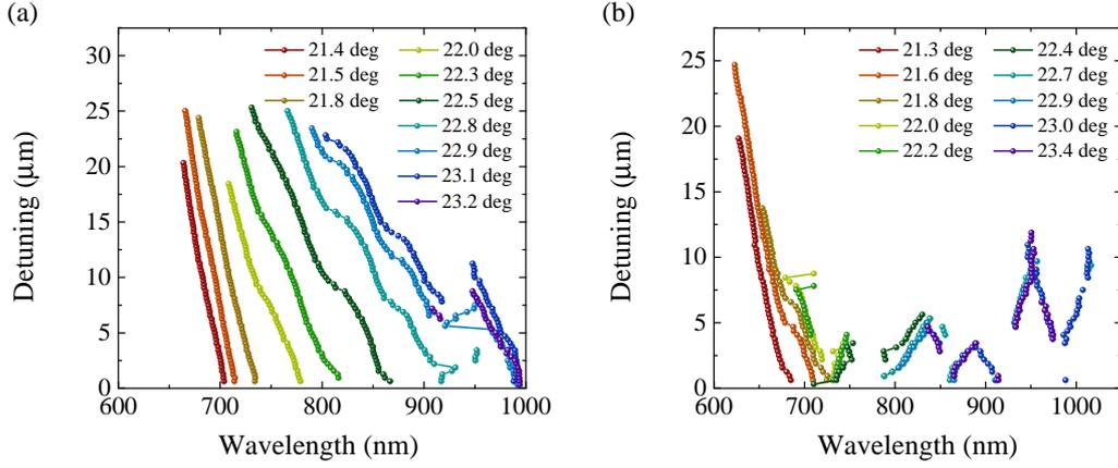
Figure 1.3 Relationship between the central wavelength of output spectra and cavity length detuning in (a) high and (b) low dispersion cases.
